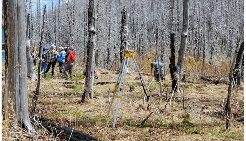
Figure 6. Students acquire hands-on experience in key considerations for using specialized GPS for locating mapping plots, including canopy, timing, and optimal location for connecting to the satellite. [Photo courtesy of Laura Chasmer, May 2023.]
