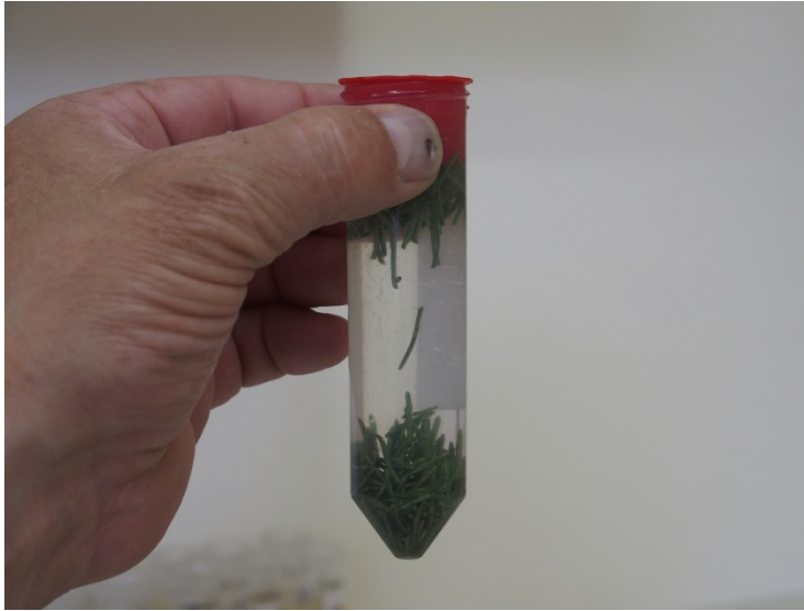
Figure 2.8 Sealed container filled with water and a tested sample (loose foliage)
