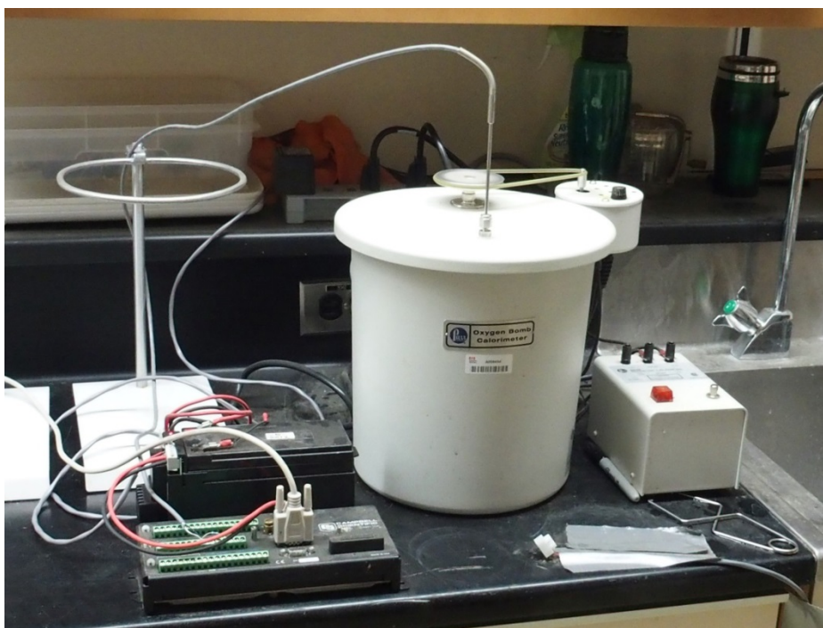
Figure 2.11 Electrical contacts for ignition of the tested sample are connected (top image); Parr model 1341 Plain Jacket calorimeter ready for the test (bottom image).
