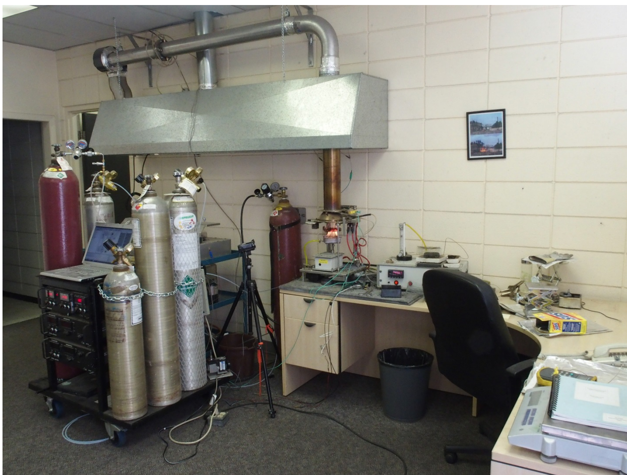
Figure 2.7 Oxygen consumption calorimeter used for the flammability testing.
