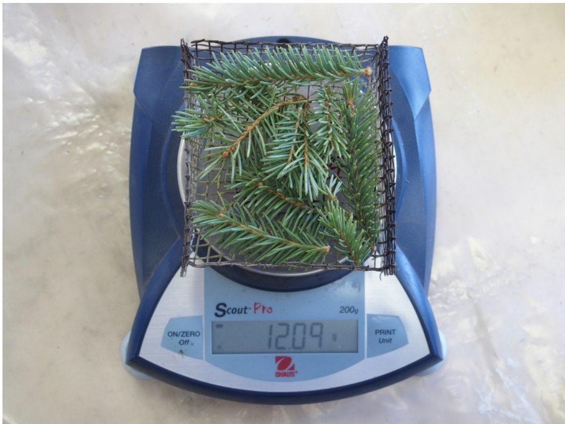
Figure 2.3 Fuel sample number 132, new shoots, fresh mass 12.09 g., sampled on September 15, 2014. The shoots were placed into a 10x10cm wire-mesh sample holder and weighed using a precision balance.
