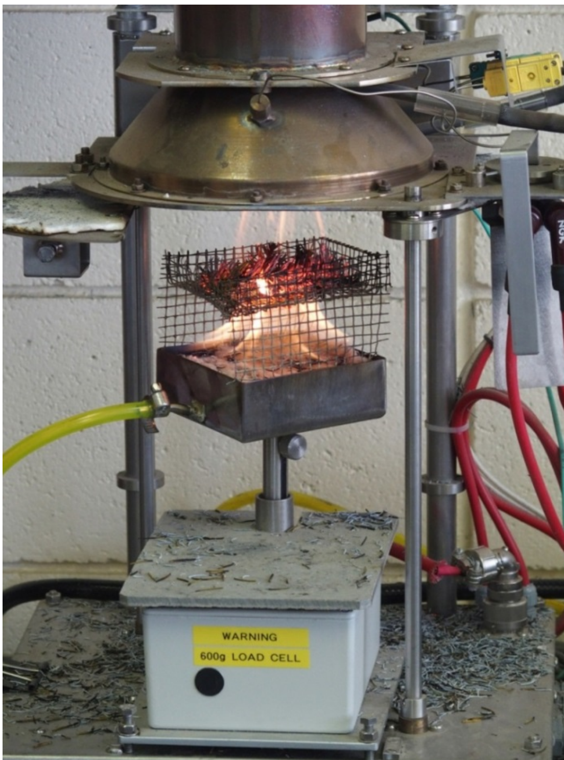
Figure 2.6 Experimental setup (from bottom to top): load cell, methane burner, incoming methane flame, wire-mesh sample holder, burning live fuel sample, outgoing flame (methane flame with the burning sample within the flame).
