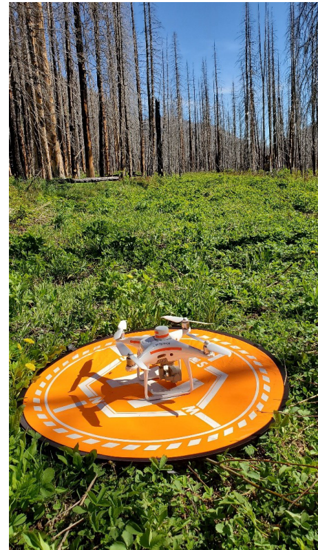
Photo by Laura Chasmer, taken in Waterton Lakes National Park, Alberta. Chasmer and Hopkinson's team uses drones with multi-spectral sensors plus photography to collect measurements in addition to complementary fieldwork and lidar.
